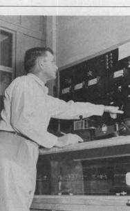
A GREAT SKILL is required to operate some of the instruments. Without it how could Harvey Skaloud calibrate a meter using the K2 potentiometer and galvanometer?
